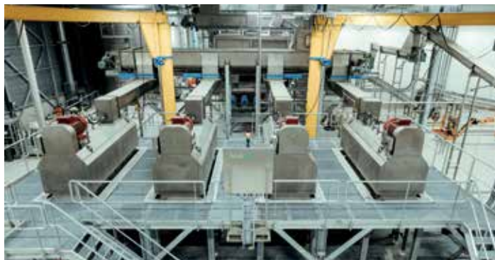
Four Paddle Depackers processing 60 tons of food waste per hour
