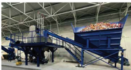
Complete food waste depackaging line at biogas plant in Romania
