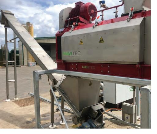
Mavitec Green Energy is specialized in food waste and depackaging solutions with short payback times, high separation efficiency and proven concepts. Our machines are designed to separate the organic material from the packaging and deliver the cleanest organic product that is extremely suitable for several purposes such as biogas installations.
