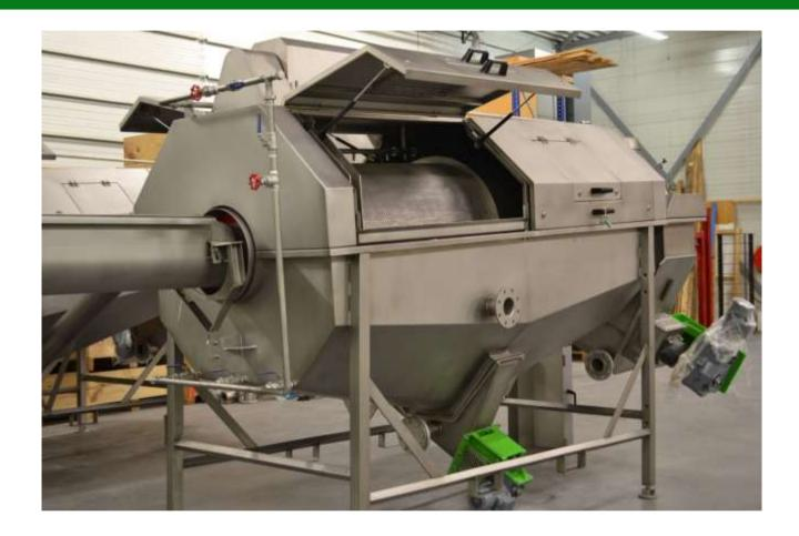
**Function:** the Washing Drum cleans the removed packaging with warm water to make it free from fats and other organic material.
