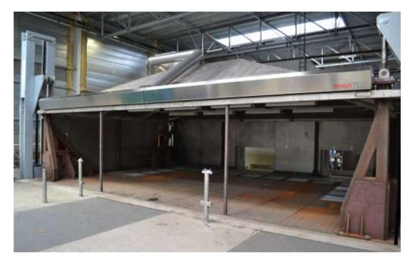
**Mavitec Green Energy** offers a unique bin for melting and separation of used cooking oils/yellow grease. The bins are executed with a heavy, hydraulic operated, moveable floor.
