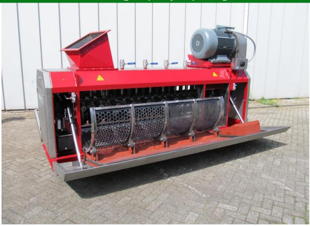
**Function:** Producing a clean organic product suitable for biogas installations by separating the organic material from the packaging.
