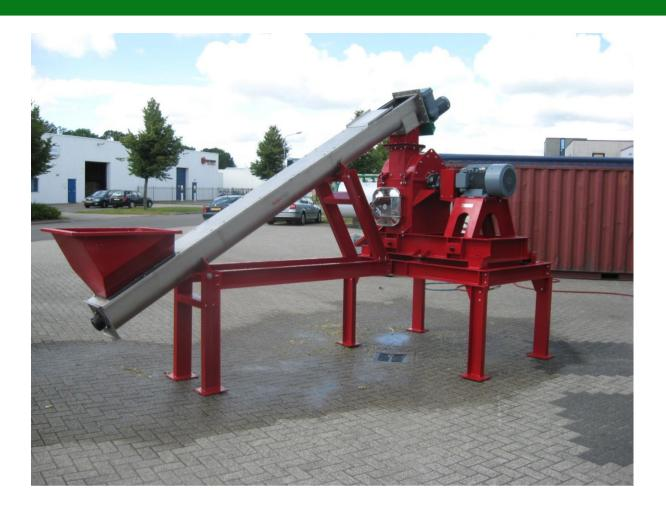
**Function:** to grind shop returns, restaurant returns and any other food products suitable for recycling and/or biogas additives.
